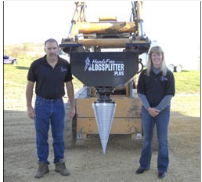
Charlie and Joni VanDusartz display their Hands-Free Log Splitter that is attached to a skid steer.
